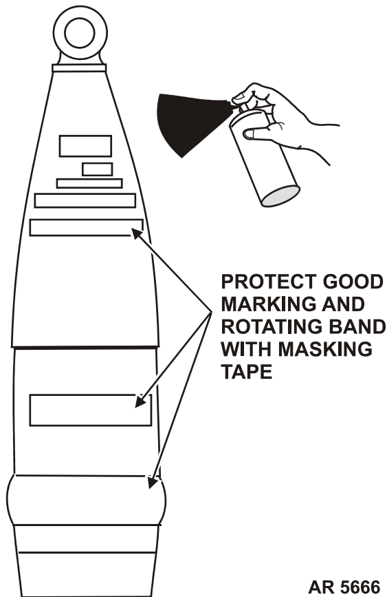
Figure 3-20. Using Spray Paint for Touchup.
